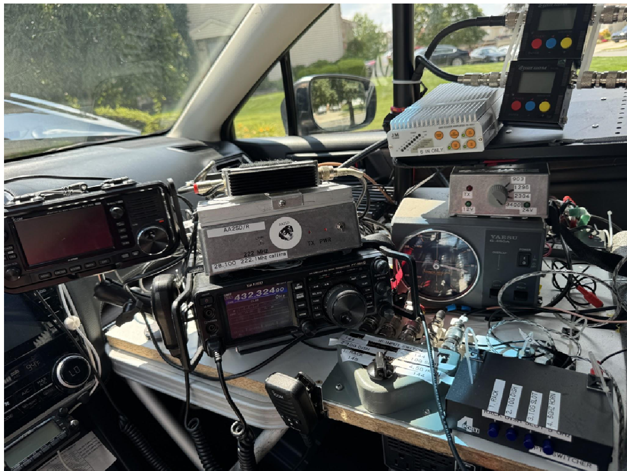
ICOM 705 mounted in my Rover Set up left of the FT991A as the IF radio for microwave.
