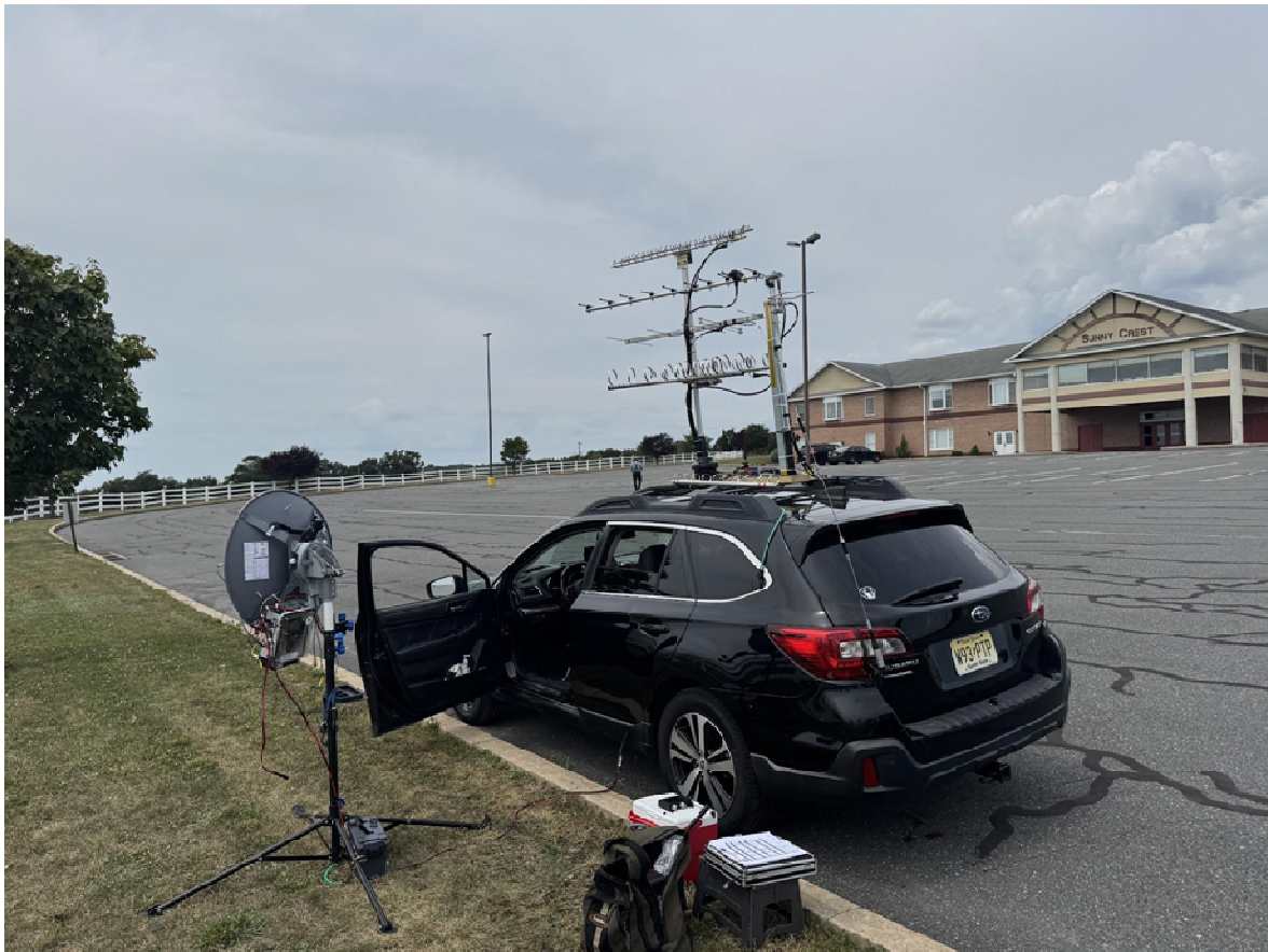
Rover Set up at FN20AD during the start of the 222 and Up contest with upgraded 222 4 Element Beam and a 10 Element 432 Yagi.
